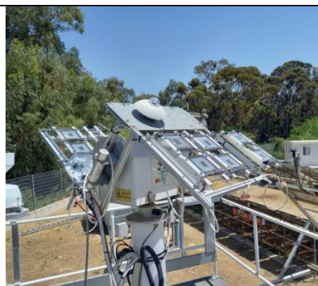
Figure 1: Perovskite mini-modules mounted outdoors on a tracker at the University of Cyprus site
